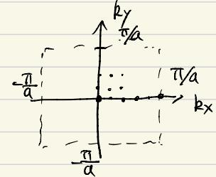
$$\vec{k} = \frac{2\pi}{L} \vec{n}, \quad n_x, n_y, \dots = -\frac{L}{2} + 1, \dots, \frac{L}{2} \quad \text{第-布里渊区}. \quad |k_x|, |k_y| \leq \frac{\pi}{a}$$
